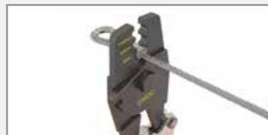
Swage the swage sleeve two times using the HS-14CR swage tool. One swage on either end of the swage sleeve is the preferred method. End of sleeve must be flush with crimping tool.
