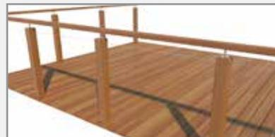
Pass the unattached end of the wire through the pre-drilled intermediate posts.
