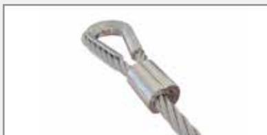
Form a loop in one end of the wire using the thimble and swage sleeve as shown. The wire should be protruding from the end of the swage sleeve approximately 2mm prior to swaging.
