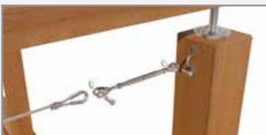
Mount the saddle to the opposite post and attach the rigging screw to the looped end of the wire and saddle as shown. Adjust bottle screw by turning middle section.
