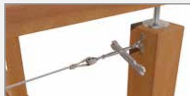
Tension the rigging screw with the ProRig c-spanner as shown to the desired tension.
