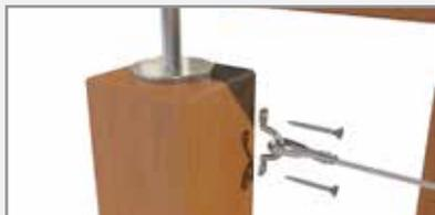
Insert the saddle through the loop and mount saddles (as per diagram) to the end post using the screws provided.
